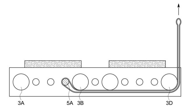
For a high starting point, redirect the band around roller 3D, and hold it in place with pin 5A. This configuration is useful for the following exercises:
