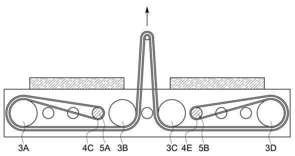
For center loading, route the band as shown. Use one or two handles, a bar or a hip belt to pull up the resistance band. Adjust the pin location as needed.
