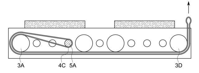
For a low starting point, redirect the band around rollers 3A and 3D. Hold the band with pin 5A, pick the location as needed for the exercise.
